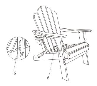
8.Use screw (6) to install the pin onto part(B)and part(C) as shown in the diagram.
