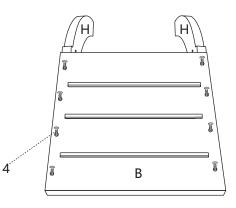
2.As shown in the figure, connect part(B) to part (H) using screw (4) .
