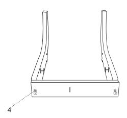
1.As shown in the figure, connect part(I) to part (H) using screw (4).
