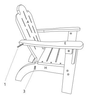
8.Attach part(A) to part (E) by using screws (1) as shown in the diagram. Attach part(A) to part (H) by using screws (3) s shown
