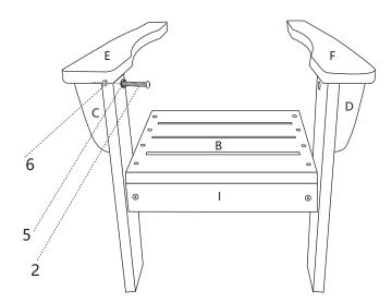
6.Attach part(E) to part (C) by using screws (2) and nut(6) and gasket(5) as shown in the diagram.
