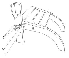
3.Attach part(D) to part (H) by using screws (2) and nut(6) and gasket(5) as shown in the diagram.
