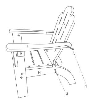
7.Attach part(A) to part (F) by using screws (1) as shown in the diagram.
