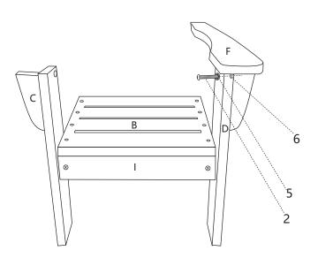
5.Attach part(F) to part (D) by using screws (2) and nut(6) and gasket(5) as shown in the diagram.
