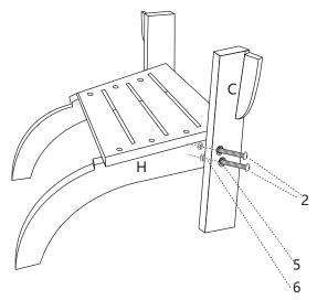
4.Attach part(C) to part (H) by using screws (2) and nut(6) and gasket(5) as shown in the diagram.
