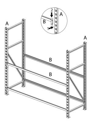
STEP 5: Repeat steps 2 through 4 to join the next set of beams at the same level to form the second shelf frame, as shown in detail #2. Note: The columns are adjustable in 3" increments. You can adjust the wire shelf shelves to any height you desire.
