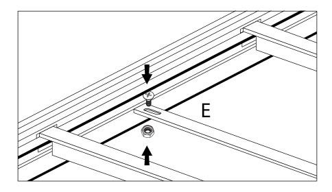
STEP 7: Take one beam brace and attach it to the assembled unit as shown in detail #4. Repeat the steps to install the rest of the braces to the rack. Make sure all braces are fully seated.
